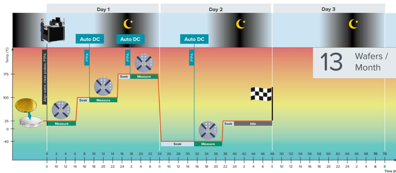
Figure 6: The CM300xi-ULN with Autonomous DC Measurement Assistant achieves a 1.8X increased wafer throughput and requires 75% less test engineers time than Figure 5.\*
