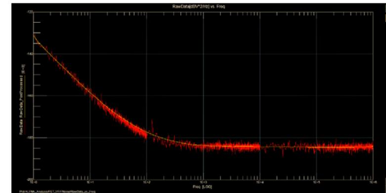
Figure 2: CM300xi-ULN chamber noise graph, 1Hz to 1MHz (VAMP LF), 32 ave, 1600points/dec, Rload and Rsource = 0 ohm, using Keysight E4727A (A-LFNA). Y-axis scale for Power -140 to -200.
