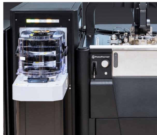
The MHU301 enables fully automated SEMI-compliant loading of up to 25 different wafers.
