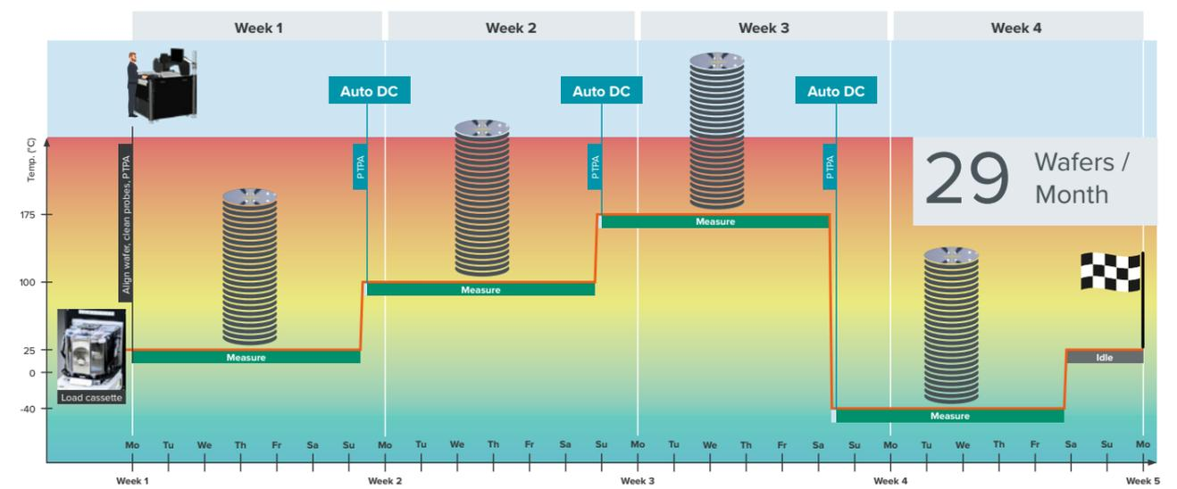
Figure 7: CM300xi-ULN with Wafer Loader MHU301 and Autonomous DC Measurement Assistant achieves 4.1X increased wafer throughput and requires 92% less test engineers time than Figure 5.\*
