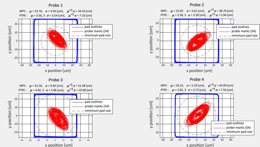
Figure 4: Measured data: 54 sets of die touchdowns / probe scrub marks, at multiple locations across 300 mm wafer, with accurate touchdown of 4 motorized probes on 30  $\mu\text{m}$  pads, at 6 different temperatures ( 25, 150, -45, 175, -55, 200°C). Conditions include wafer soak 3 hr, die soak: 10 min, and 30 min contact test time.
