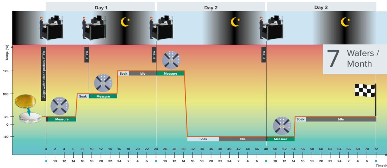
Figure 5: CM300xi-ULN with manual probe-to-pad alignment. The system is idle at night and the weekends.\*
