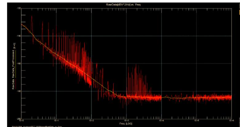
Figure 3: CM300xi-F chamber noise graph, same test conditions and display scales as both figures 2 and 3.
