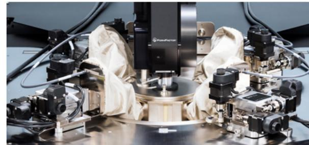
Motorized positioners with patented FlexShield.
