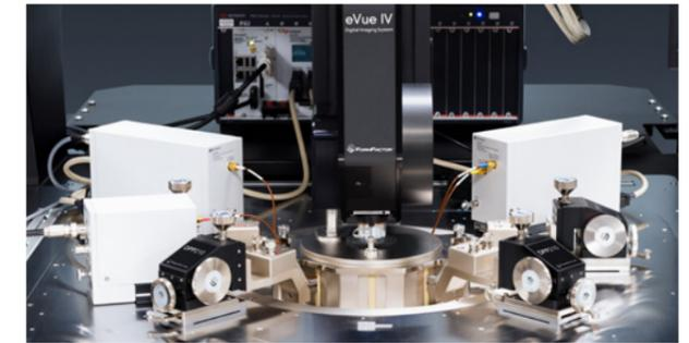
Figure 1: Test setup for chamber noise data using Keysight E4727A (A-LFNA). Three DCP-HTR probes connected to drain, source, gate terminals. All probes inside the probe station MicroChamber shielding environment.
