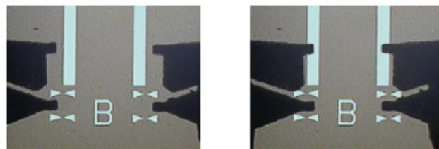
**Figure 2:** Images showing correct alignment and placement of probe tips
